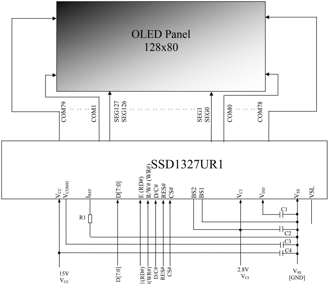
Voltage at I<sub>REF</sub> ≈ V<sub>CC</sub> - 3V.
