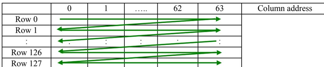
When A[2] is set to 1, the driver is set to vertical address increment mode. After the display RAM is read / written, the row address pointer is increased automatically by 1. If the row address pointer reaches the row end address, the row address pointer is reset to row start address and column address pointer is increased by 1. The sequence of movement of the row and column address point for vertical address increment mode is shown in Figure 10-3.
