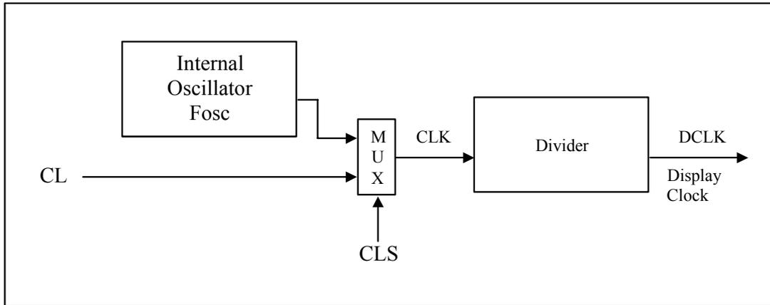
The display clock (DCLK) for the Display Timing Generator is derived from CLK. The division factor “D” can be programmed from 1 to 16 by command B3h.
