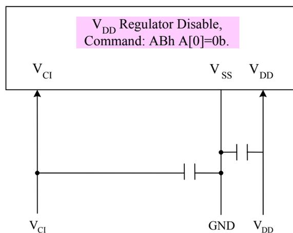
No RAM access through MCU interface when there is no external / internal V<sub>DD</sub>.
