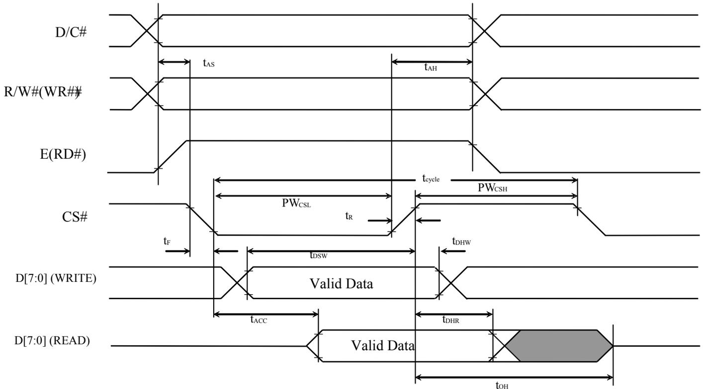
Table 13-3 : 8080-Series MCU Parallel Interface Timing Characteristics
