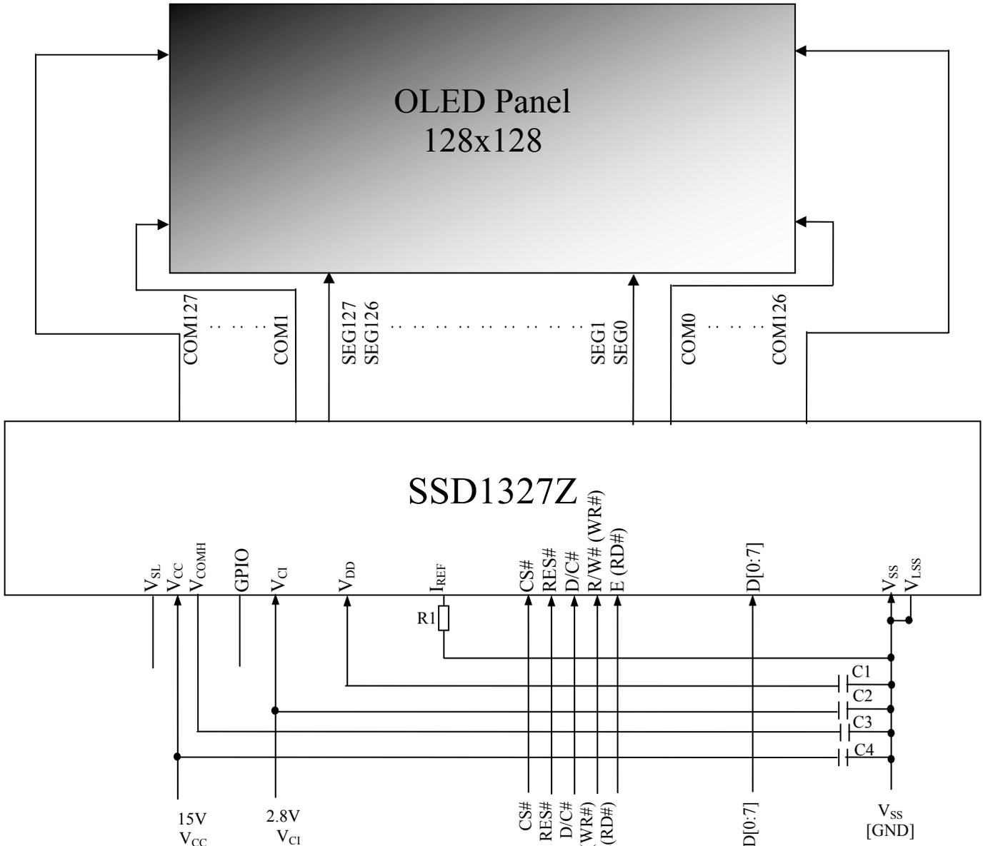
Voltage at  $I_{REF} \approx V_{CC} - 3V$ . For  $V_{CC} = 15V$ ,  $I_{REF} = 10\mu A$ :
